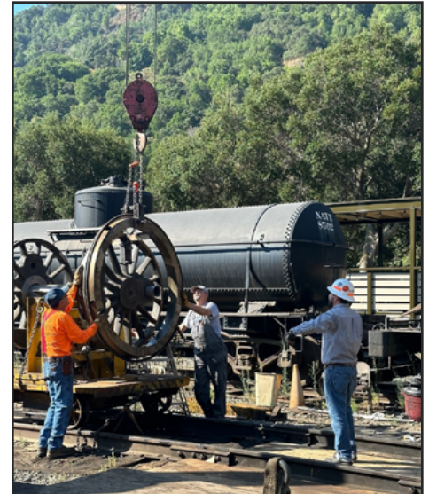
Volunteers position a new tire for installation on one of the locomotives 6 driving wheel centers.
