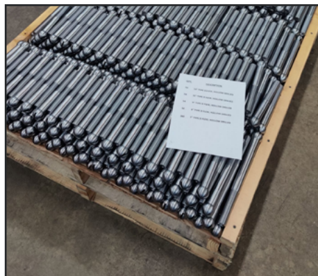
Newly machined Flexible Staybolts, ready for installation, funded in part by our generous donors.
