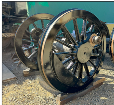
Drive Wheels, complete with new tires and new paint, ready for reinstallation.
