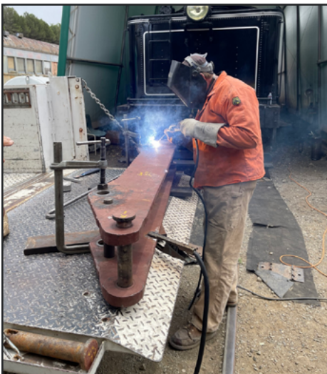
Volunteer welder John Blaine welds a spring pack back together after repairs.
