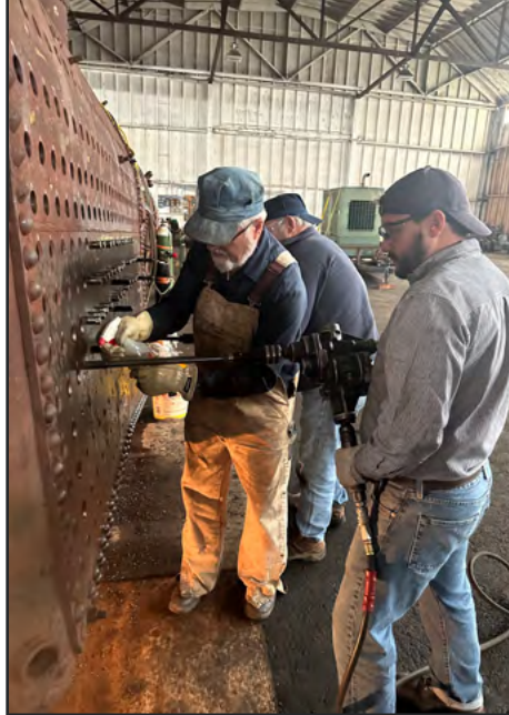
Alan Siegwarth Photograph Chuck Kent reaming holes in the back, Henry Chandler and Charles Franz tapping staybolt holes.
