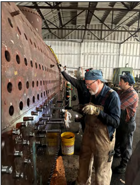
Alan Siegwarth Photograph Henry Chandler threading staybolts in with Dylan Olson and Stathi Pappas in the background.
