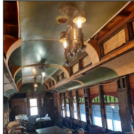
Lights in the 2nd class section. Hard to grasp, but this is only half the car. The 330 is a 69' car of wood construction with iron rods on trusses. Last of the composite car era.
