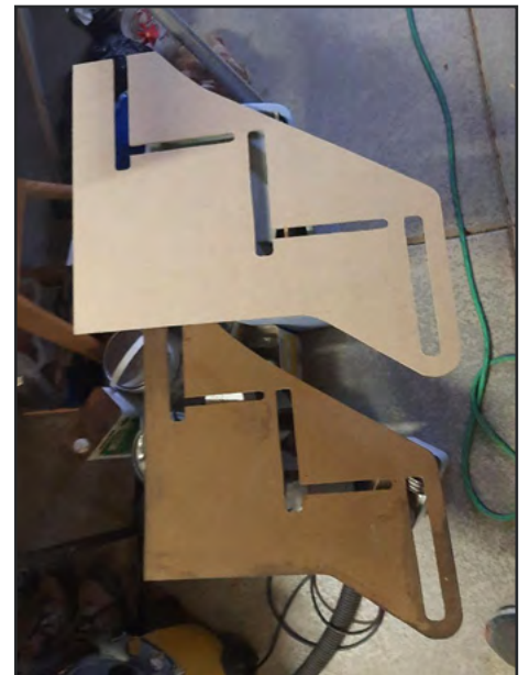
Pattern for step side bracket with old one below. That 3" gained will make all the difference when loading passengers at both ends.
