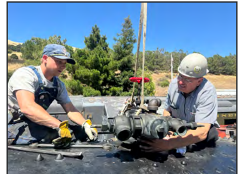
Alan Siegwarth photograph Scott Kennedy and John Blaine mounting the turret back on top of the #2479.
