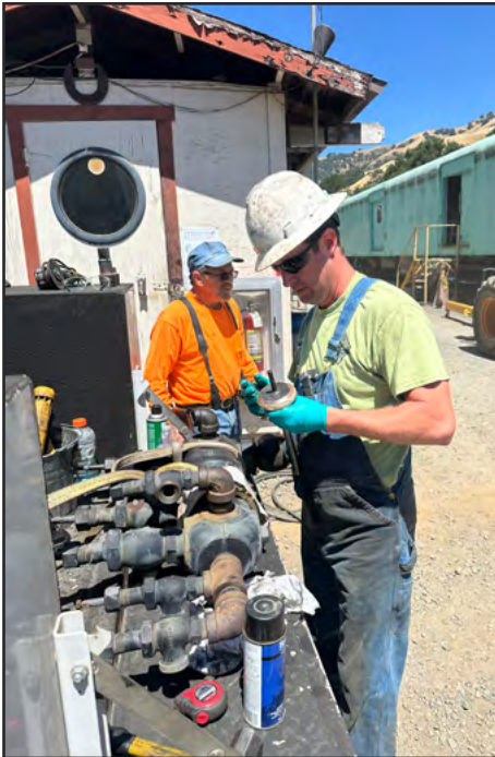
Alan Siegwarth photograph Chris Brophy lapping valves on the turret in preparation for a hydrotest.
