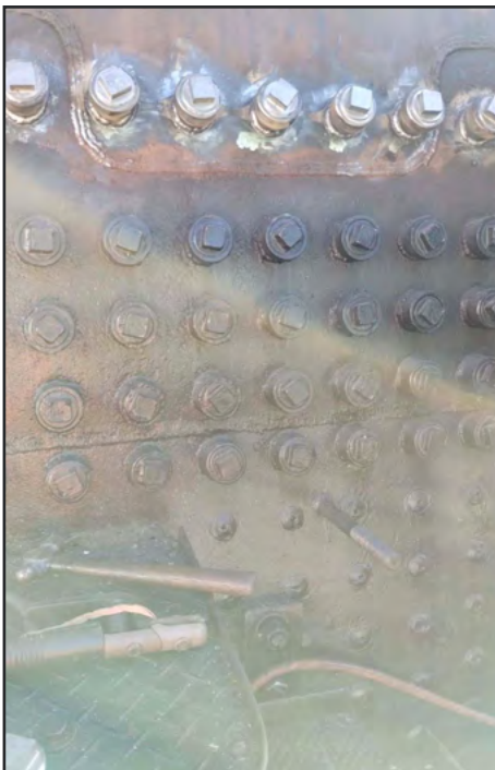
Chuck Kent photograph Lower row of sleeves and flexible stays installed.
