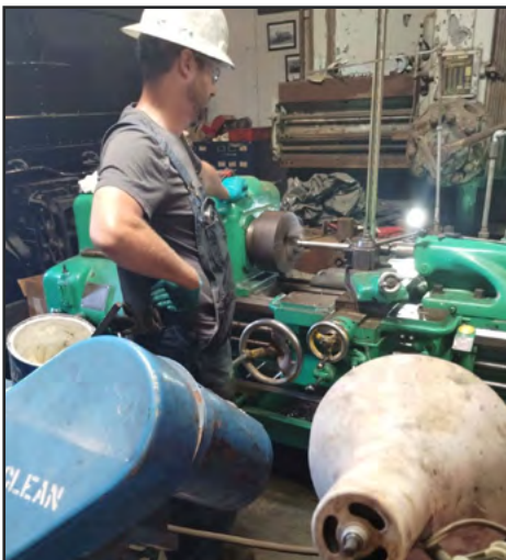
Chuck Kent Photograph Chris Brophy machining a staybolt to fit.
