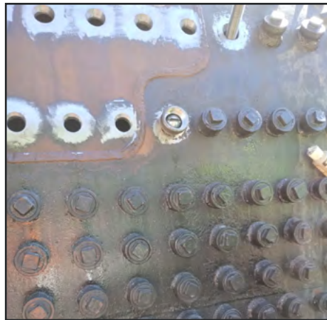
Alan Siegwarth photograph Patch progress picture with one sleeve welded on and the flexible staybolt installed in the center of the picture.
