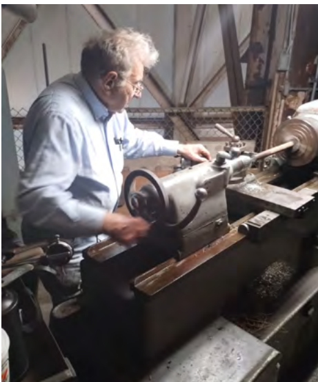
Chuck Kent Photograph Art Randall using the lathe upstairs that he repaired to operate again to turn a staybolt.
