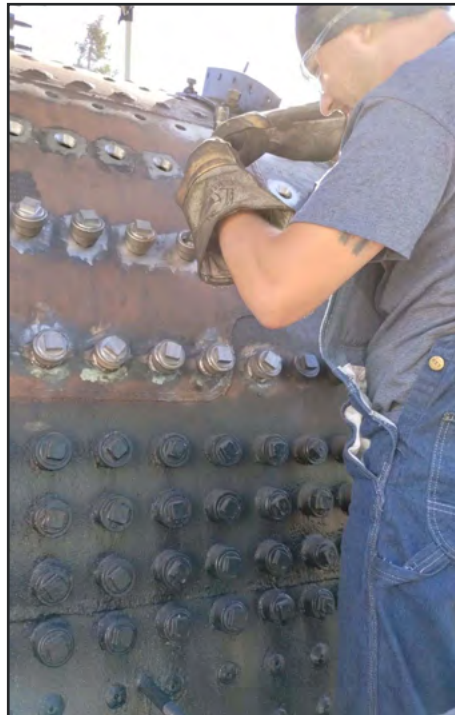
Chuck Kent photograph Scott threading a flexible stay in place.
