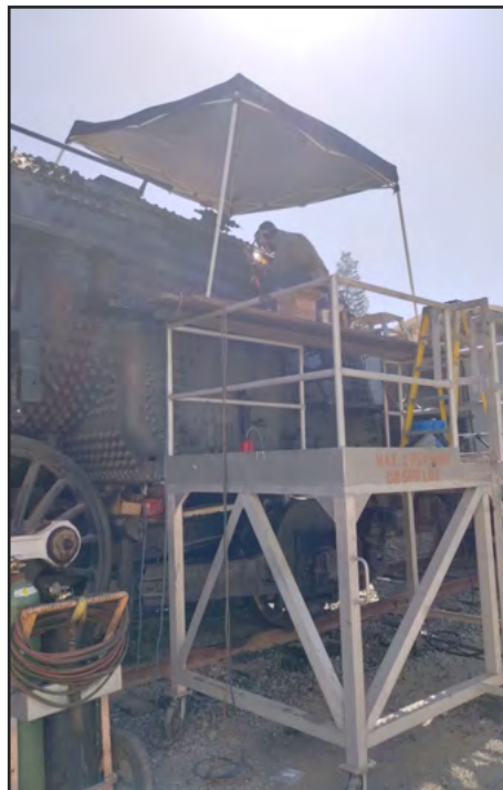
Chuck Kent photograph Scott Kennedy at work welding sleeves in place.
