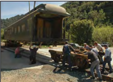
PLA volunteers use the Armstrong method to roll the rear truck under the 330.
