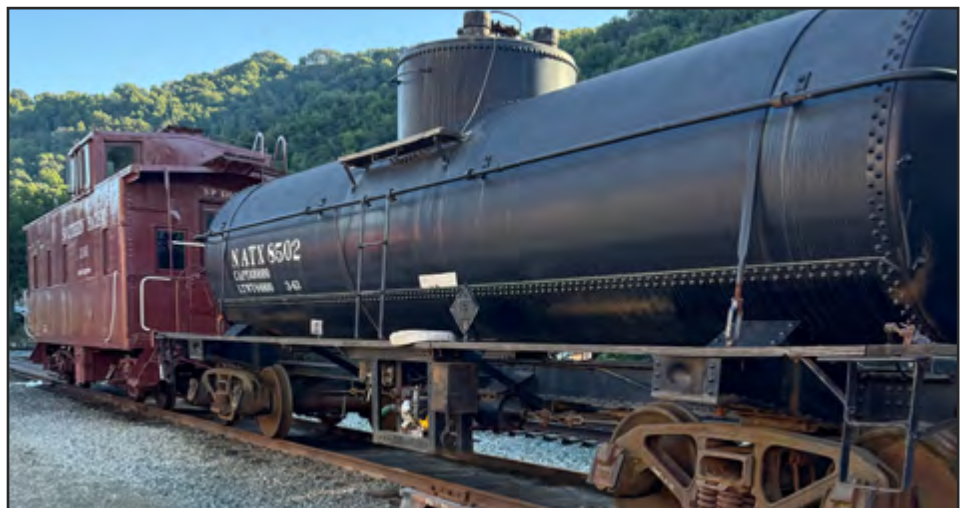
Tank car picture shows in-mounted pump that allows the tank car to provide water to fill our steam engines.
