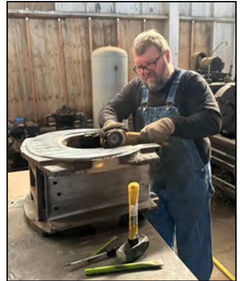
Alan Siegwarth photograph John Gradden working on cleaning up the driving boxes after pouring the babbitt thrust bearing.
