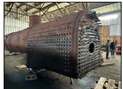
Stockton Locomotive Works photograph Overall view of the boiler and substantial amount of staybolt work completed.
