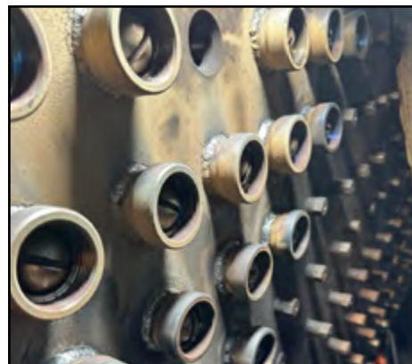
Stockton Locomotive Works photograph Flexible staybolt sleeves welded in place after installation.
