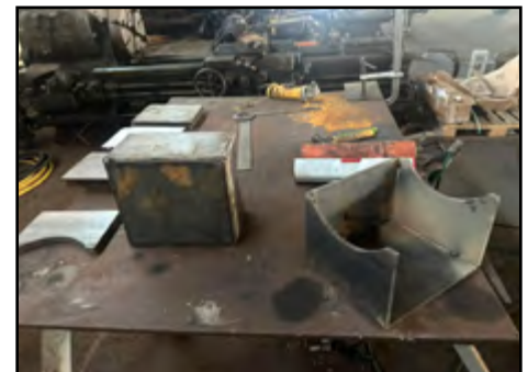
Alan Siegwarth photograph New oil cellars in the process of being fabricated by SLW.
