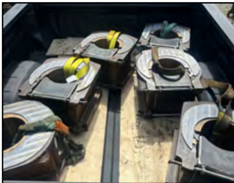
Newly machined driving boxes and cellars arrive at Brightside.
