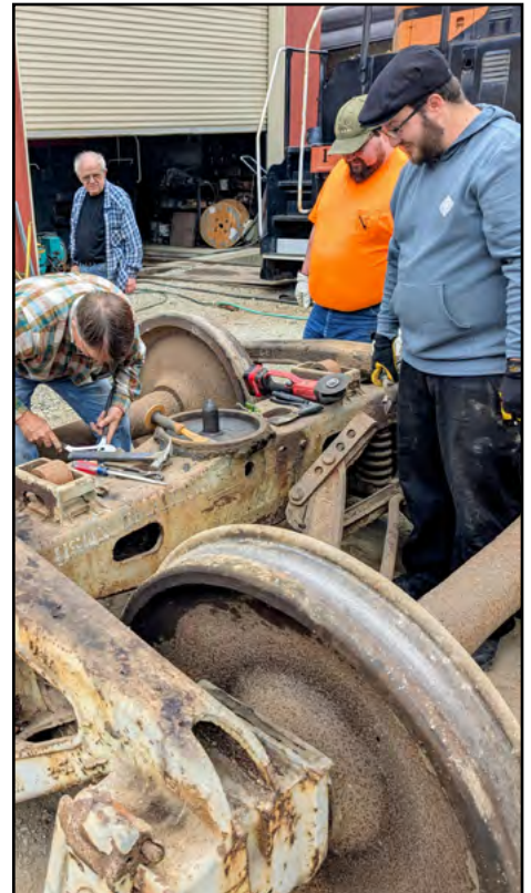
Stephen Barkkarie photograph Garon, Mason, Howard and Bill supervise the repair to a truck from under the Navy Boxcar.
