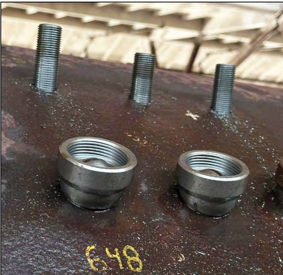
Stockton Locomotive Works Photograph View of crown and flexible stays installed on the outside of the boiler. Stockton Locomotive Works.
