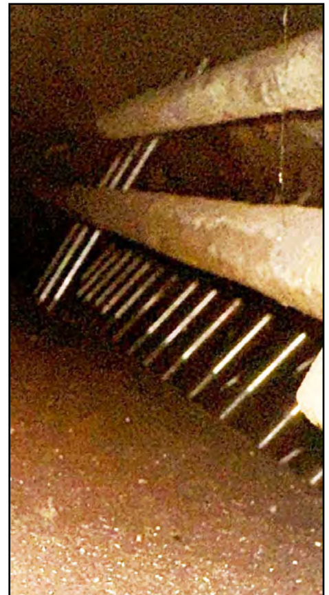
Stockton Locomotive Works photograph Crown stays installed in the SP #1744 boiler with more to be done.
