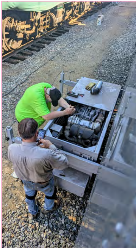
Stephen Barkkarie photograph Rich Alexander and Doug Vanderlee locate fault in Stadco generator.
