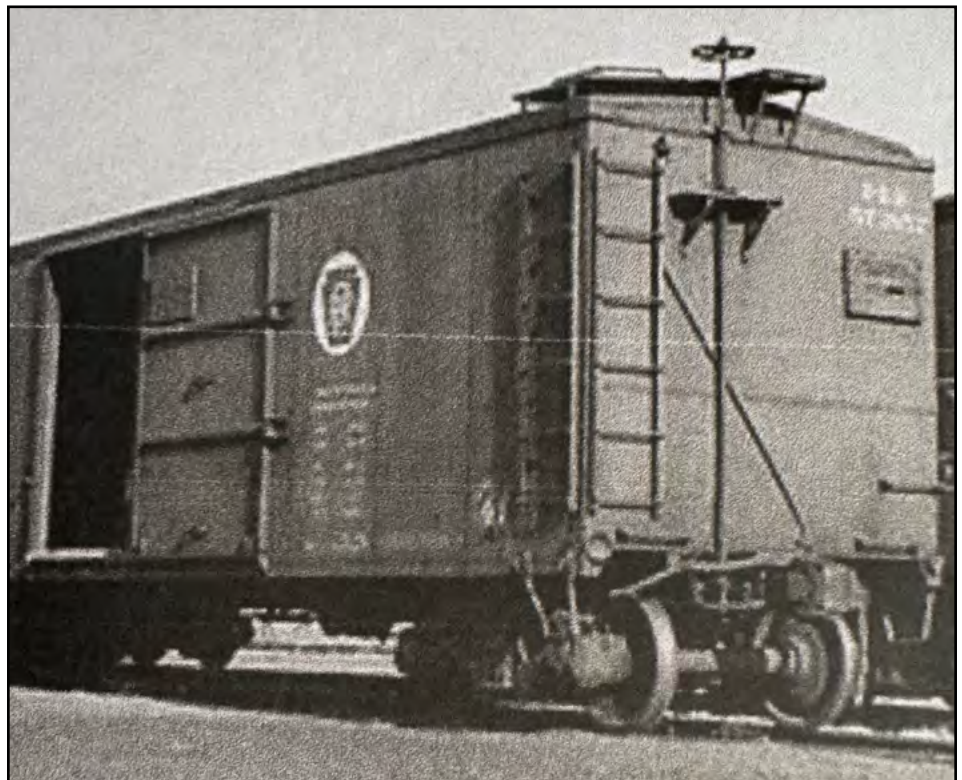
Another X-29 boxcar before upgrade on doors. Sides and ends converted to steel.
