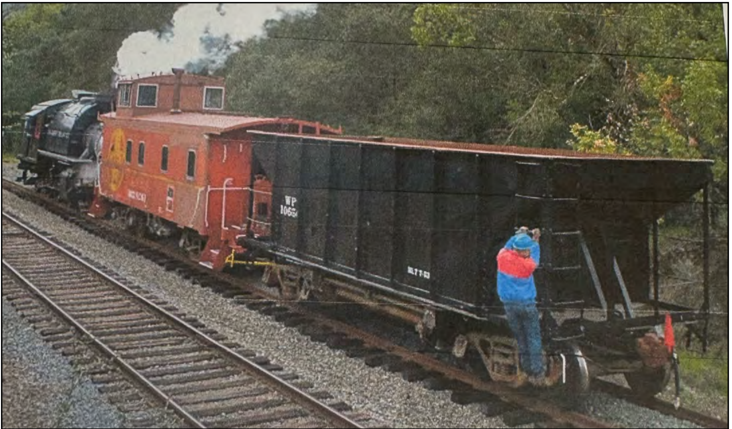
Here is hopper WP 10656 laying down ballast on NCRY.
