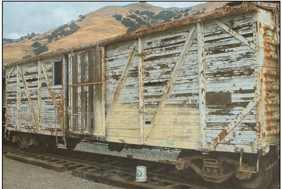
This car is a B-50-16 with its slated wood sides and steel braced supports and Dreadnaught ends. Not perfect, but still hanging in there.
