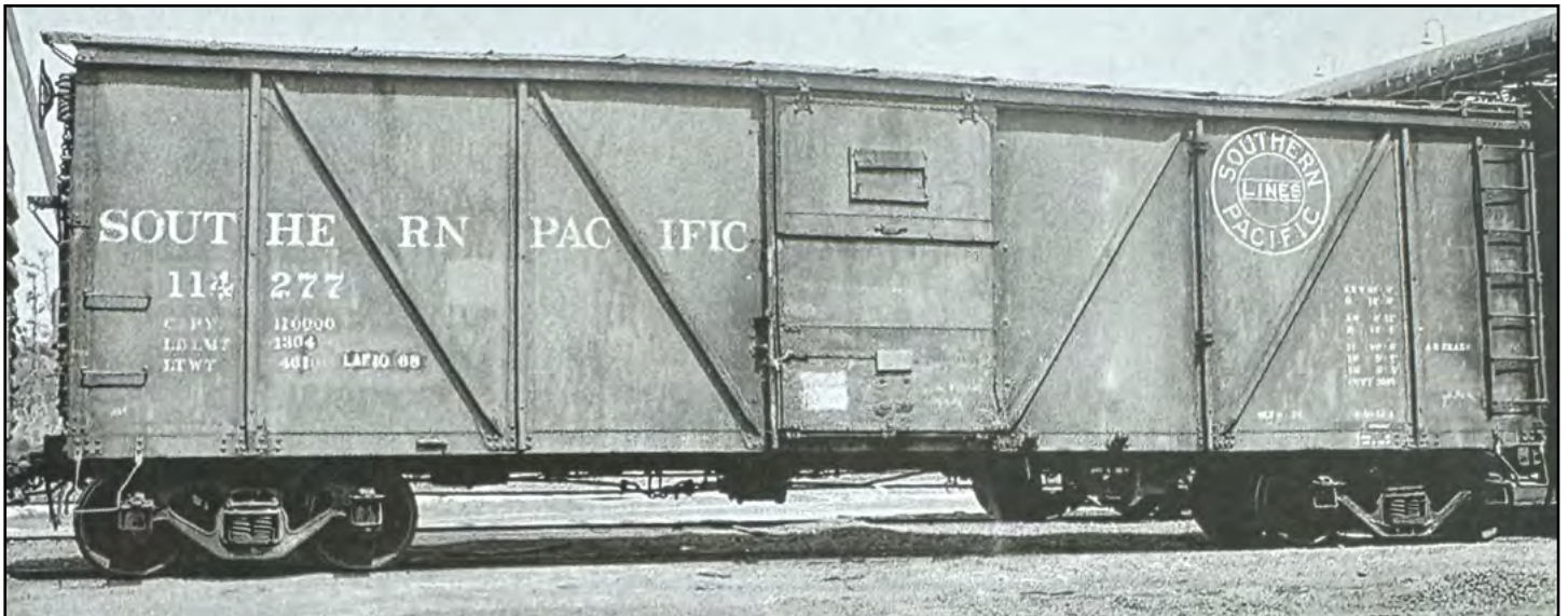
This is a B-50-15 in its new steel sides with the outside brace supports.
