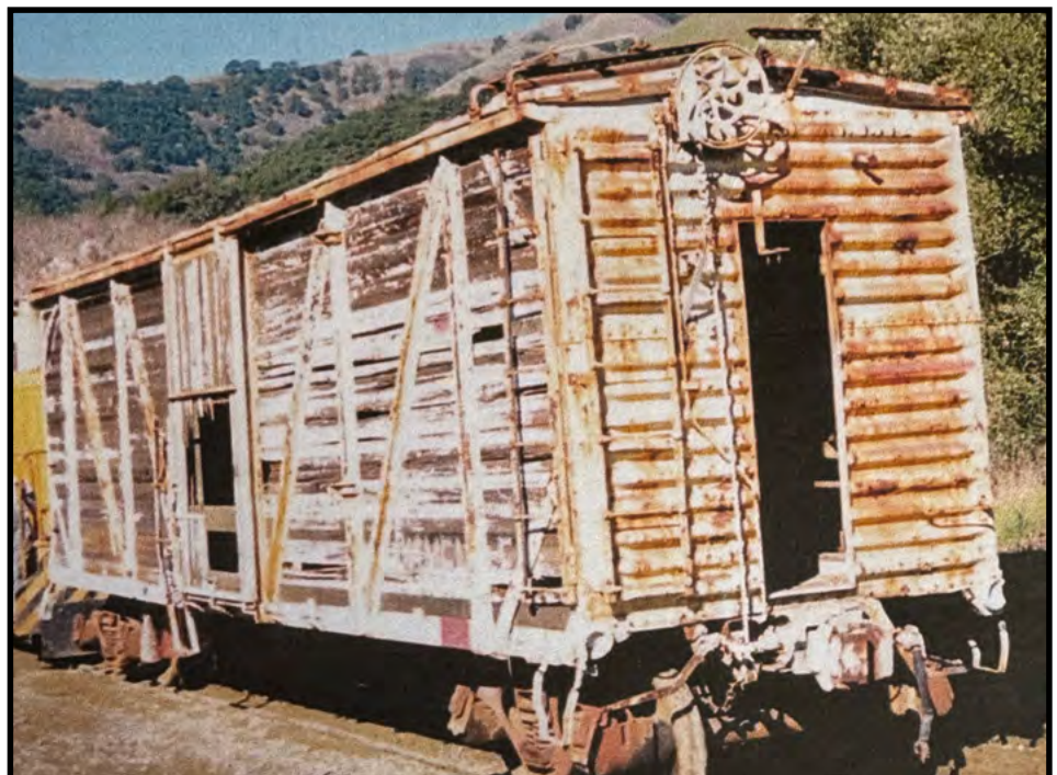
This is the car at the Spot with wood removed. This B-50-16 is ready for a rebuild.
