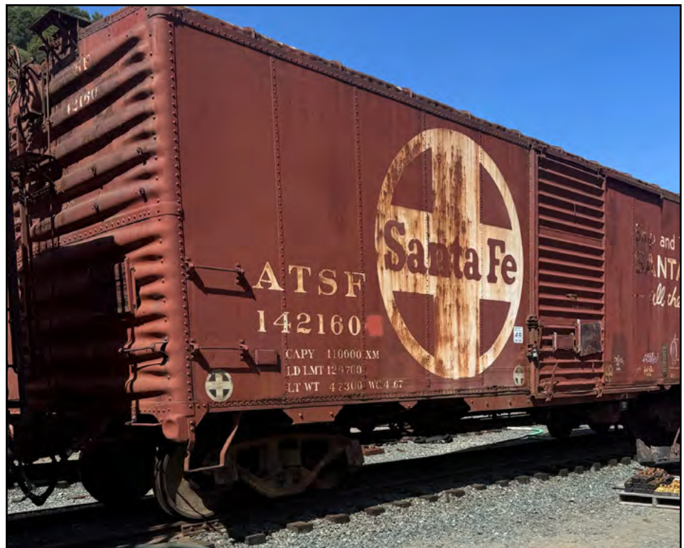
Picture of a BX-37 boxcar with B-1 trucks.
